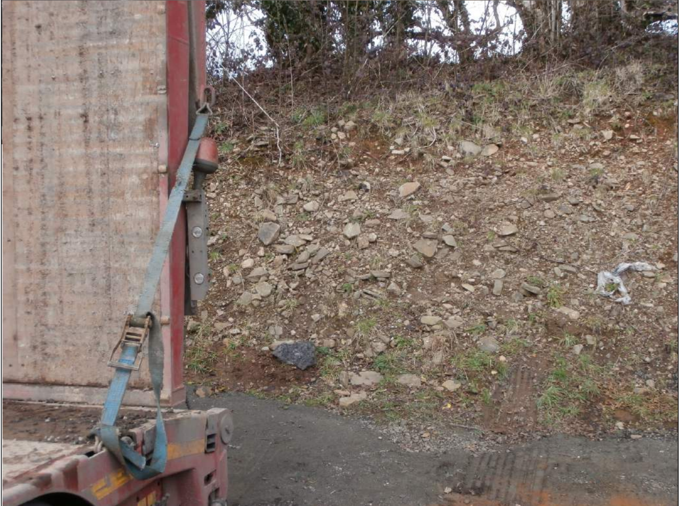
FIGURE 11 (TOP) CUT IN GLACIAL TILL IMMEDIATELY SOUTH EAST OF THE SITE FIGURE 12 (BELOW) CLOSE UP OF MATERIAL SHOWING LARGE, ANGULAR PENNANT SANDSTONE COBBLES AND BOULDERS
